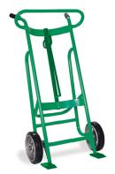
2-Wheel EZY-Rol™Automatic Drum Trucks feature ValleyCraft's exclusive EZY-Tilt™ design and spring-loaded chime hook so the operator never has to touch the drum. Choice of steel or aluminum. Shoes adjust to handle 30- and 55gal. drums up to 1,000 lbs. Available with optional hand brakes for added safety. Replaceable wheels, shoes and axles available. Five-chime hook and three-wheel options available.
