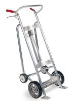
4-Wheel EZY-Rol™ Automatic Drum Trucks are available in steel or spark resistant aluminum and feature ValleyCraft's exclusive EZY-Tilt™ design and spring-loaded chime hooks. Operator never has to touch the drum. Trucks handle 30and 55-gal. drums up to 1,000 lbs. Available with optional hand brakes. Models feature replaceable wheels shoes and axles. Five-chime hook and 3-wheel options available.
