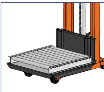
**R-5 Roller Bed:** Excellent for transferring heavy objects to and from a lift with minimum effort. Front or side loading. Rollers are on a 3" center. 27 x 30" area mounted on a 32 x 36" slip-on platform. 1000 lb capacity, weight is 145 lbs. Requires a 24" load center.
