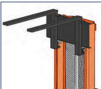
**Reversed (Inverted) Forks:** Ideal for overhead installation. Forks can be modified in a reverse position, giving an increased lowered/raised height.
