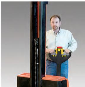
Narrow mast and offset design provide workers a clear view with no blind spots.
