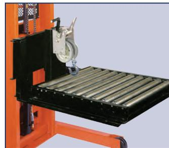
**P-6 Die Puller:** Equipped with a hand operated winch with cable and hook for pulling dies over a roller bed. 27 x 30" roller area mounted on a 32 x 30" slip-on platform. 1000 lb capacity, weight is 185 lbs. Requires 24" load center.
