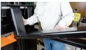
Adjustable fork carriage allows forks to be repositioned to best accommodate loads (straddle only).
